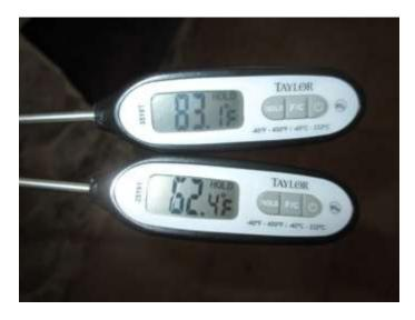
Repair needed: The air conditioning mode on the second-floor did not appear to be operating properly at the time of the inspection. In the A/C mode the supply air was  $68.5^{\circ}$ ; the return air was  $85.1^{\circ}$  for an operating differential of  $16.6^{\circ}$ . The normal operating differential range is between  $14.0^{\circ}$  and  $20.0^{\circ}$ .
